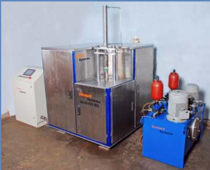
INSMART CIP installed at NML, Jamshedpur Capacity: 75mm dia x 150mm height
