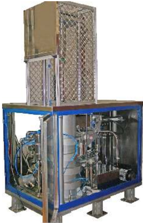
INSMART CIP installed at LASTEC, Delhi Capacity 100mm dia x 450mm height
